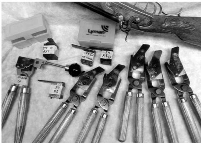
*A lineup of bullet molds presently owned by the author, some of which have been used for 30 years or more. Shown are molds for: .54 caliber round ball, .56 caliber round ball, .50 caliber round ball, .50 caliber maxi ball, plus .36 and .44 caliber round ball and conical bullet molds for percussion revolvers, along with two molds for .41 Remington Magnum bullets. The author currently owns 17 guns he casts bullets for, 11 of which are muzzleloaders.*
