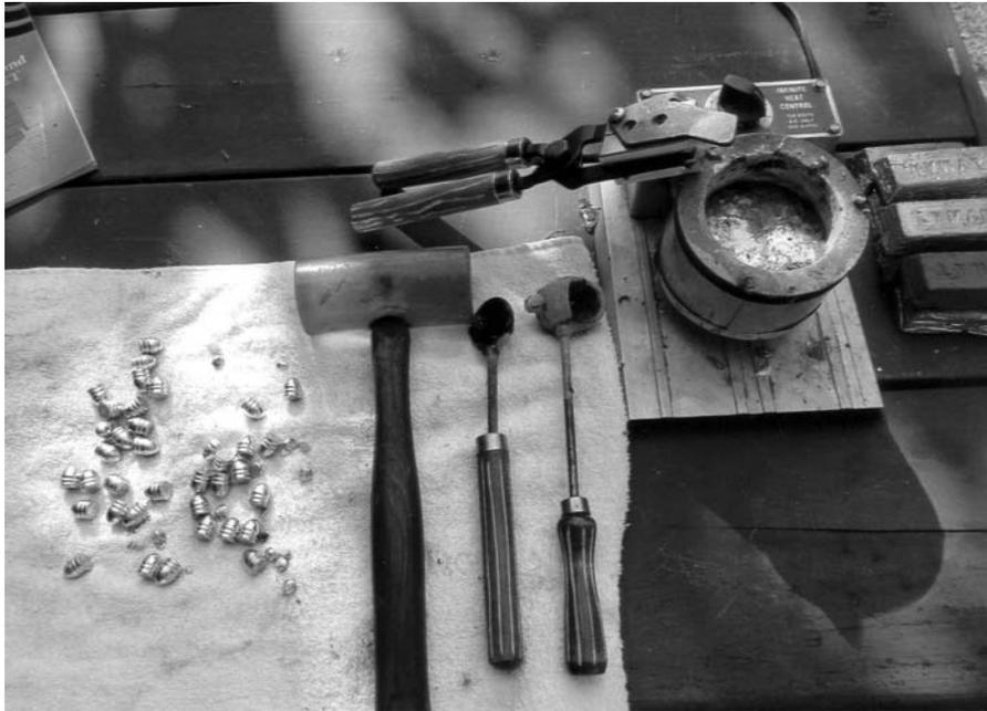
*The makings for casting bullets: an electric furnace, bullet molds, tools, and a supply of lead. Why buy bullets when for a small investment you can make as many as you want?*
