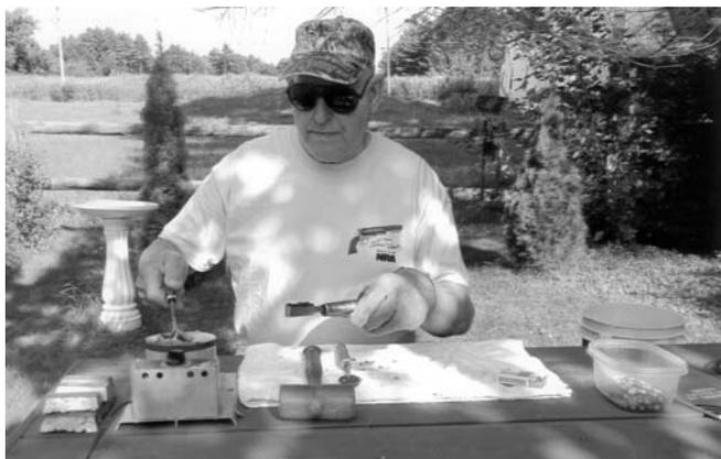
*Using a 2 cavity mold such as shown here, the author can set up and cast a hundred bullets in less time than it takes to go out and buy them – if the retailer even has them to sell! And, the cost is usually zero. Gloves are optional – eye protection is a must.*
