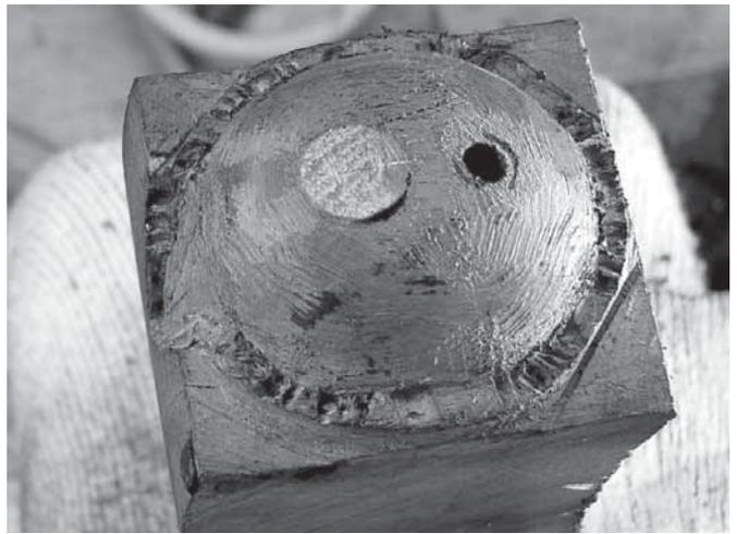
**Fig. 10** – Many little indents are now visible in the ledge around the globe as well as points of interference that need to be removed.
