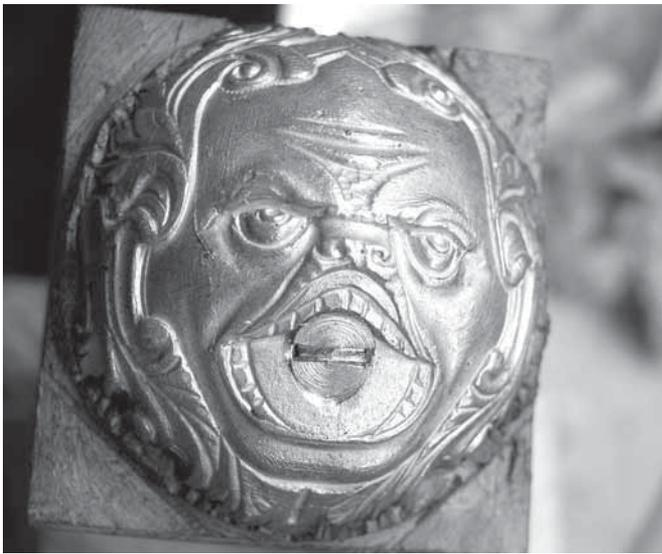
**Fig. 9** – This screw is the sole means of butt cap attachment (other than the close inleting). The screw head has been reduced to allow sufficient clearance past the teeth.
