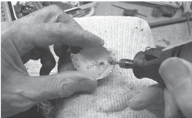
Fig. 2 – Removing the heavy casting lug from inside the thin shell of the cap was a delicate operation.
