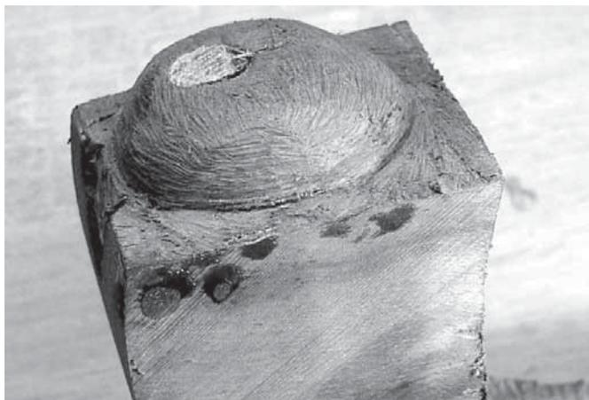
Fig. 7 – At this stage, the globe of wood is rough-shaped to allow the cap to start settling into place.
