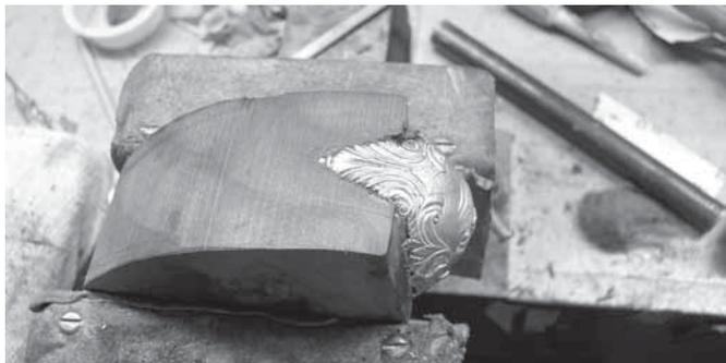
Fig. 12 – The return has been inlet flush with the wood surface. A thin layer of wood will be removed to allow the raised areas of the casting to stand a bit proud.
