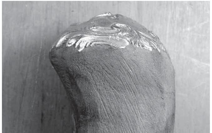
**Fig. 11** – The cap is now in place with no noticeable gaps. It will still take a lot of final sanding, polishing and a bit of engraving to fill out some of its features.
