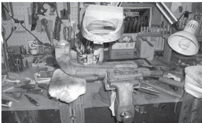
Fig. 13 – This adjustable rest, like the cantilevered lighted magnifying lens, was invaluable during the inletting process. The second lamp was used for oblique lighting to shadow imperfections in the inlet.
