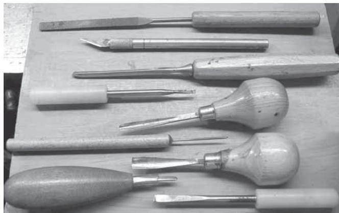
Fig. 14 – The tools used in the inletting are pretty standard items that are necessary for rifle carving and inletting.
