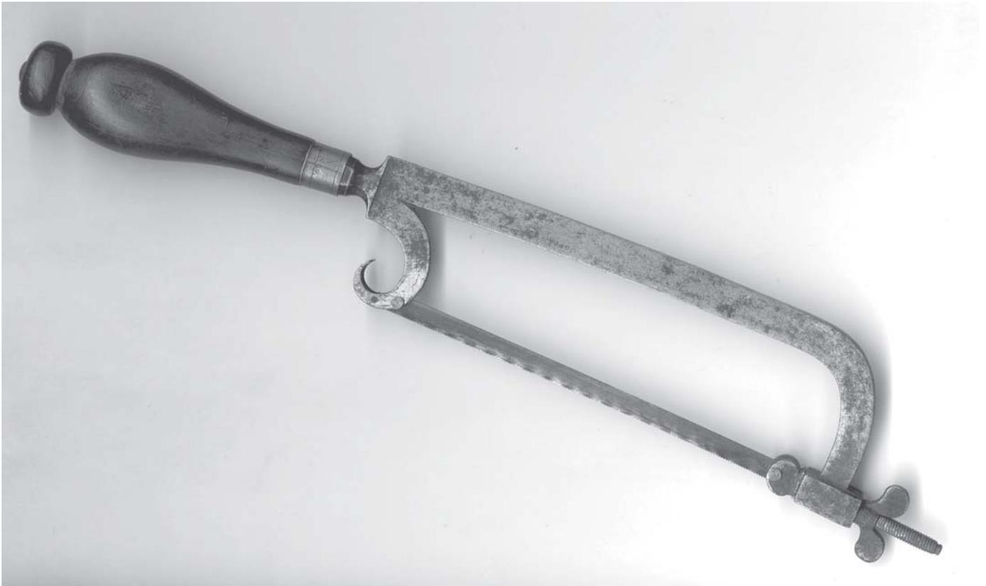
Photo 6 – Small hacksaw – this saw is small and sweet; it is fitted with a 5x 1/4" blade right off the tool store shelf.
