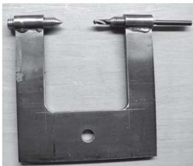
(Fig. 14) If you don't have a drill press, this little homemade jig will do the same thing.
