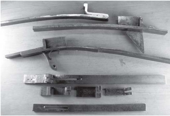
(Fig. 4) This collection of triggers and plates includes (from top) a plate hammer-forged in the traditional way by folding and unfolding to allow cutting of the slots with a saw. Next is a plate with a trigger blank. Below that is a cast trigger/plate assembly with plate extensions on both ends. At the bottom are parts for making trigger plates.
