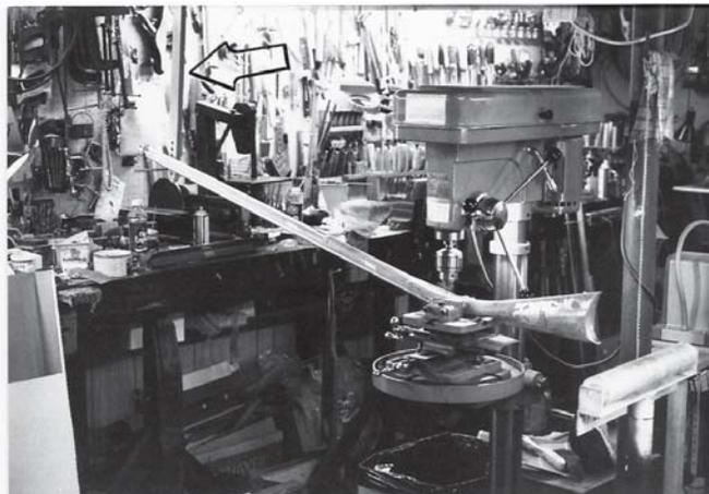
*(Fig. 10) The muzzle end of the rifle must be supported when milling out the trigger mortise on the drill press. A swinging support can be hung from the ceiling (arrow) or a roller rest can be used (seen at right).*
