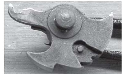
(Fig. 16) An indent ground into the belly of the lock tumbler allows a little more room for the sear to rotate and let its arm contact the trigger blade to avoid trigger rattle when the lock is at rest.
