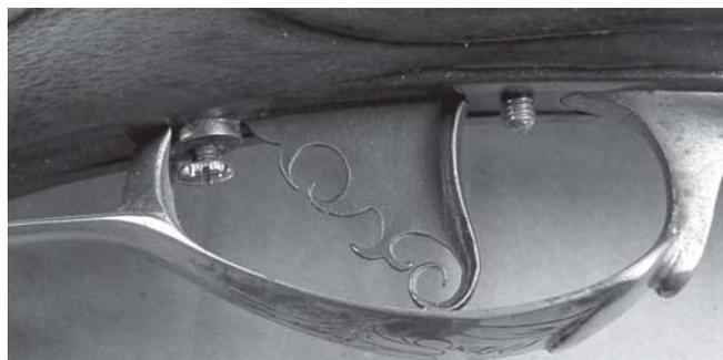
(Fig. 3) The simple single trigger allows some room for homegrown creativity. This trigger was shaped from 1/16" thick mild cold-rolled sheet metal.
