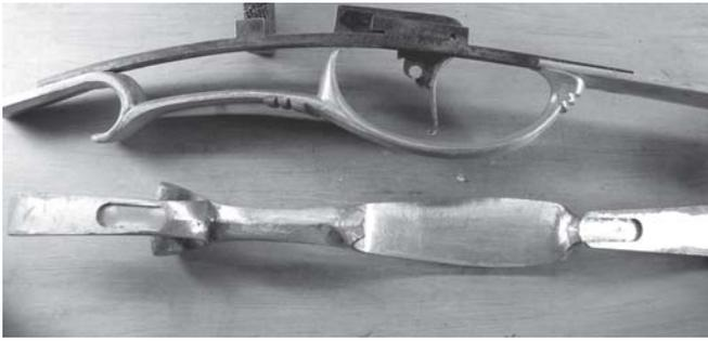
(Fig. 6) If the trigger plate is long enough, its ends can be attached to the trigger guard returns. I used to mill my trigger plates full length (top) and allow a boss to hold a light return spring to hold the trigger blade away from the sear at rest. However, I silver solder the trigger boss on now to raise the pivot point and increase leverage.
