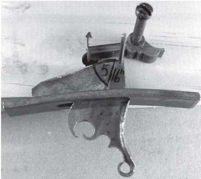
(Fig. 8) This crude mock-up shows the interaction of a simple single trigger with the sear bar of the lock. The closer the bar/trigger contact is to trigger pivot point, the easier the trigger pull. Likewise, the higher the blade is pinned in the stock, the easier the pull.
