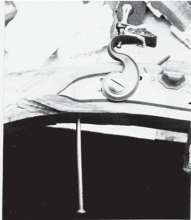
*(Fig. 9) Before you inlet your trigger, you can make a trigger “pushrod” by drilling a hole up under the sear bar and inserting a nail to trip the lock.*
