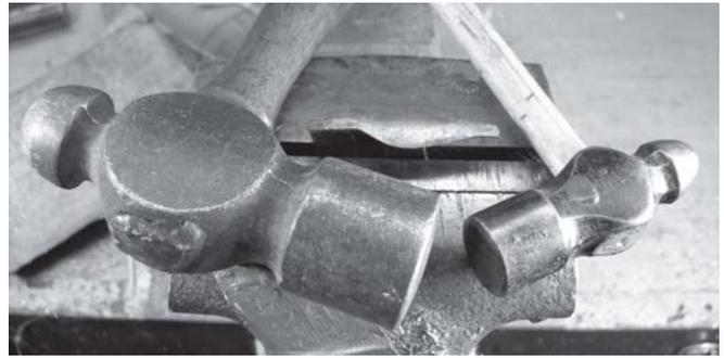
(Fig. 5) The only tools needed to shape your own single trigger are a couple of ballpeen hammers and a vise to hold the material.
