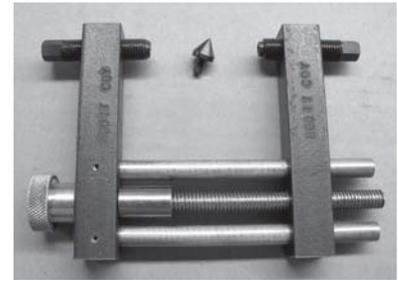
(Fig. 15) Scott Coy's alignment jig is much more sophisticated than mine. It has guides for #8 and #10 bits and a movable center point - a nice piece of work.
