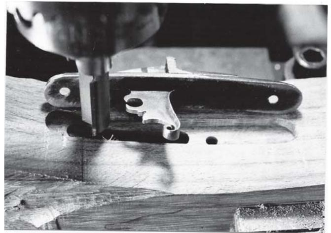
*(Fig. 12) This milled mortise will be an easy cleanup fit for the trigger assembly.*
