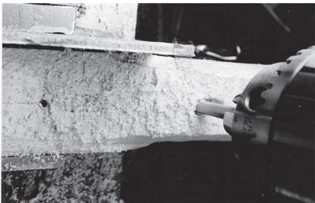
*(Fig. 11) Milling the mortise produces a mass of chips that will hide your reference lines. An assistant with a vacuum source is a big help here.*
