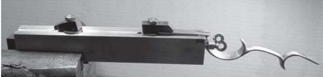
(Fig. 7). This fixture has been made from a scrap of aluminum bar. For milling indents, it can hold guards of any size from a child's rifle (shown) up to musket size guards.
