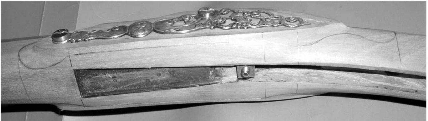
*Fig. 11 – These locator lines will help to keep the lock panel and the sideplate panel as symmetrical as possible. I bolt my trigger plate and guard together as a unit, so I spread some AcraGlas™ under the forward return to stabilize it against the pull of the lock bolt.*
