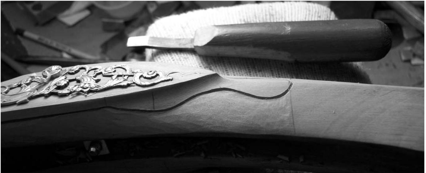
*Fig. 6 – Even under bright oblique light, a good tool will level the background to the point where little sanding is required*
