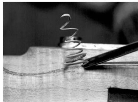
**Fig. 5** – The shape and length of the chip will tell you if your veining tool is cutting with the grain of the wood.
