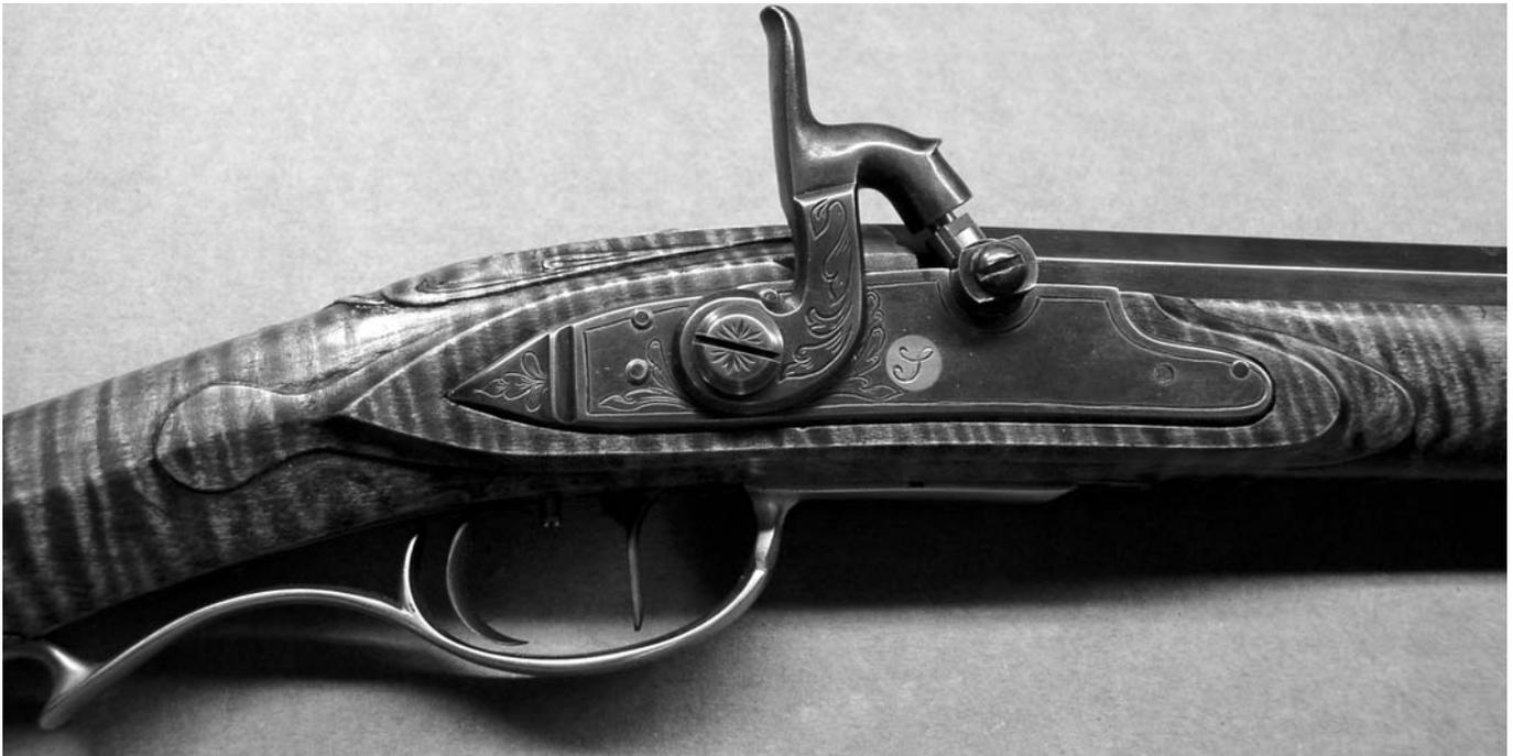
*Fig. 12 – Moldings around the lock panel of this little girl's rifle lead the eye forward and back to create a slenderizing effect.*
