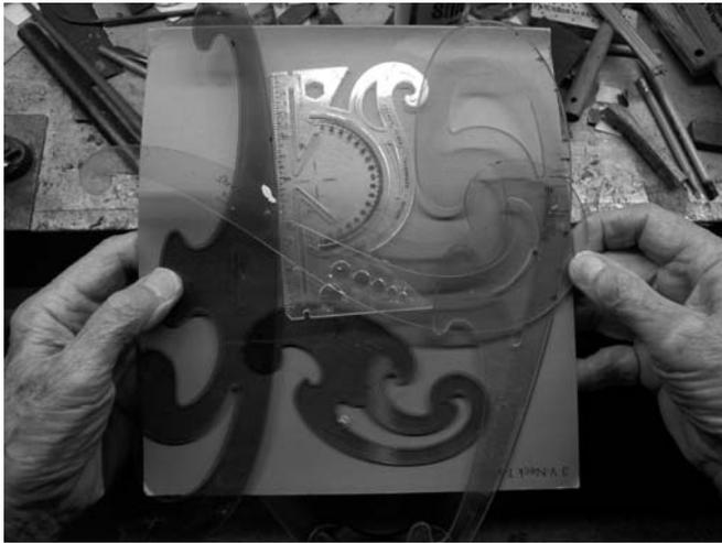
**Fig. 3** – My collection of French curves can be used to trace any molding, either directly or from a paper pattern.
