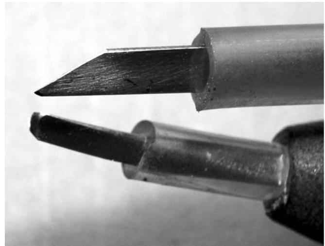
**Fig. 4b** – The veiner, like the graver, has a "heel" beveled into the belly of the tool. The graver (upper) requires only a tiny heel because it makes a relatively shallow cut into the metal and can negotiate tight curves. The veiner cuts a deeper, wider path that requires a more authoritative heel for control of the cut.
