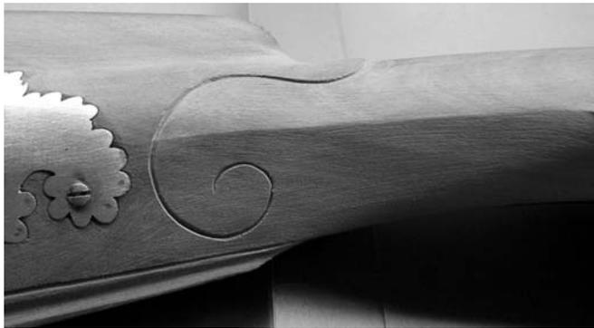
**Fig. 9** – On the lock side of the wrist, the molding can end in a bit of a decorative scroll or continue down to integrate with the curvature of the trigger guard.
