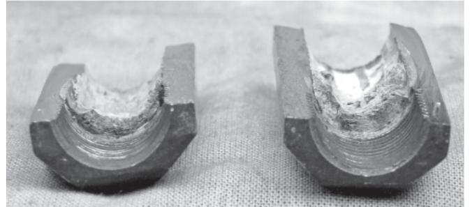
The extra ten minutes of soaking the breech area with water or other solvent, then scraping/wiping the breech plug face would prevent the problem altogether.
